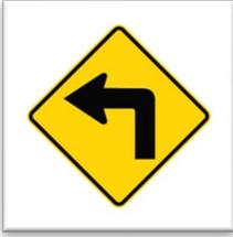
Warning sign (see graphic) would be more appropriate in this location to notify motorists of the 90-degree turns. DPD will work with the LPD sign department for installation of these signs.
